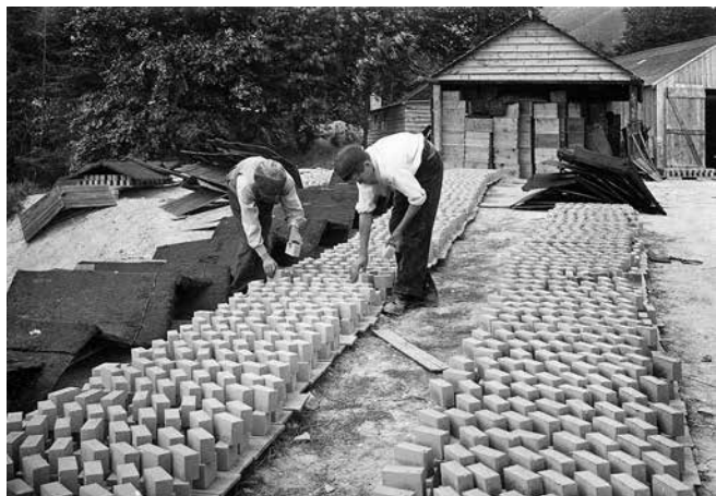
Colley Hill hearthstone factory c1910. Here, slabs of stone are being cut into small blocks instead of moulded. Completed blocks were taken by cart to a railway siding to the west of Reigate Station for transport to London
